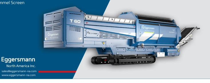
The Eggersmann T 60 is designed for customers with particularly high production requirements. It offers the remarkably precise separation efficiency typical of all Eggersmann screens with a screening capacity of up to 265 cy per hour. This makes it a high-class mobile screening solution.
