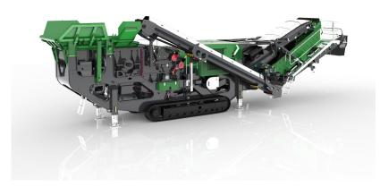
The I44R features a large impact chamber with a 4-bar rotor and a 45.6" x 32" feed opening. This design enables excellent crushing performance and ensures consistent product shape and size.
