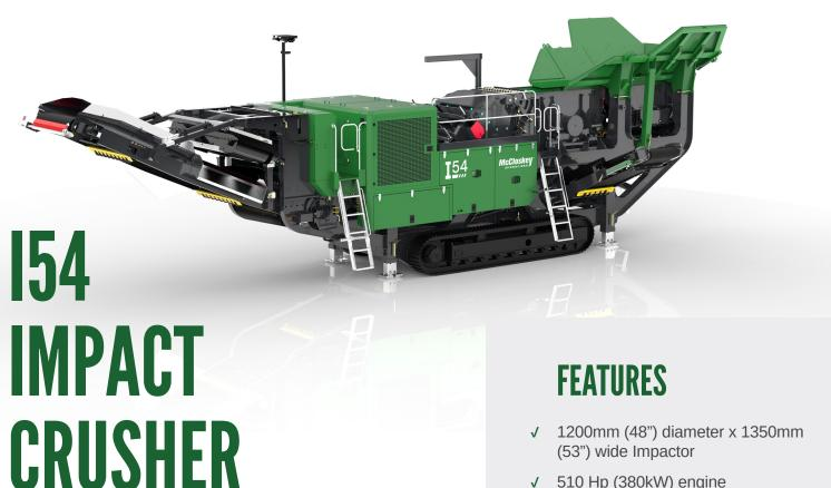
The McCloskey® I54 impact crusher is designed to deliver high levels of productivity and efficiency. It is equipped with a large impactorallowing it to handle a wide range of materials effectively.
