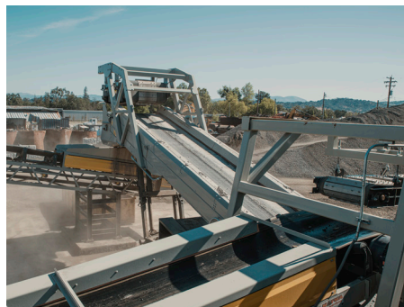
Set up for recycling applications, the conveyor features reinforced belting, special wear alloys, and a vibrating pan feeder.
