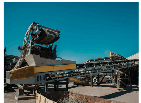
Lippmann's self-cleaning electro magnet makes quick work of removing metal debris, ensuring your operation runs smoothly and efficiently.
