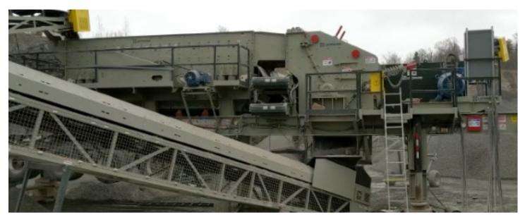
The 5165i-ws is a secondary impact crushing plant perfectly suited to be paired up with a primary jaw crusher. The screen plant and impactor are perfectly paired to size the material for your required specification. The impactor is heavy-duty enough to handle recycle material and will withstand the tramp metal that might be present from the primary crusher. The top cross conveyor is extended to ensure you can take both products out on the same side of the plant.
