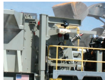
On-board jib crane simplifies blow bar replacement process for ease of maintenance.
