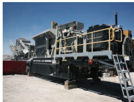
This self-contained impactor plant is equipped with a direct drive 415hp (310kW), Tier 4 Final engine.
