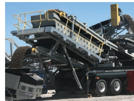
Hydraulically adjustable screen angle allows you to select the appropriate angle for your application. The spreader split ensure material is evenly deposited on the vibrating screen.
