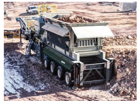
Rugged Lippmann feeder is capable of handling side or rear loading from various types of equipment.
