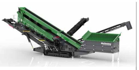
The benefits of dual screenboxes are endless. You are in control of each box separately, allowing you to dial in the stroke, speed and direction for each box independently. Also, the overall machine weight is lighter with two boxes, as compared to one large box.
