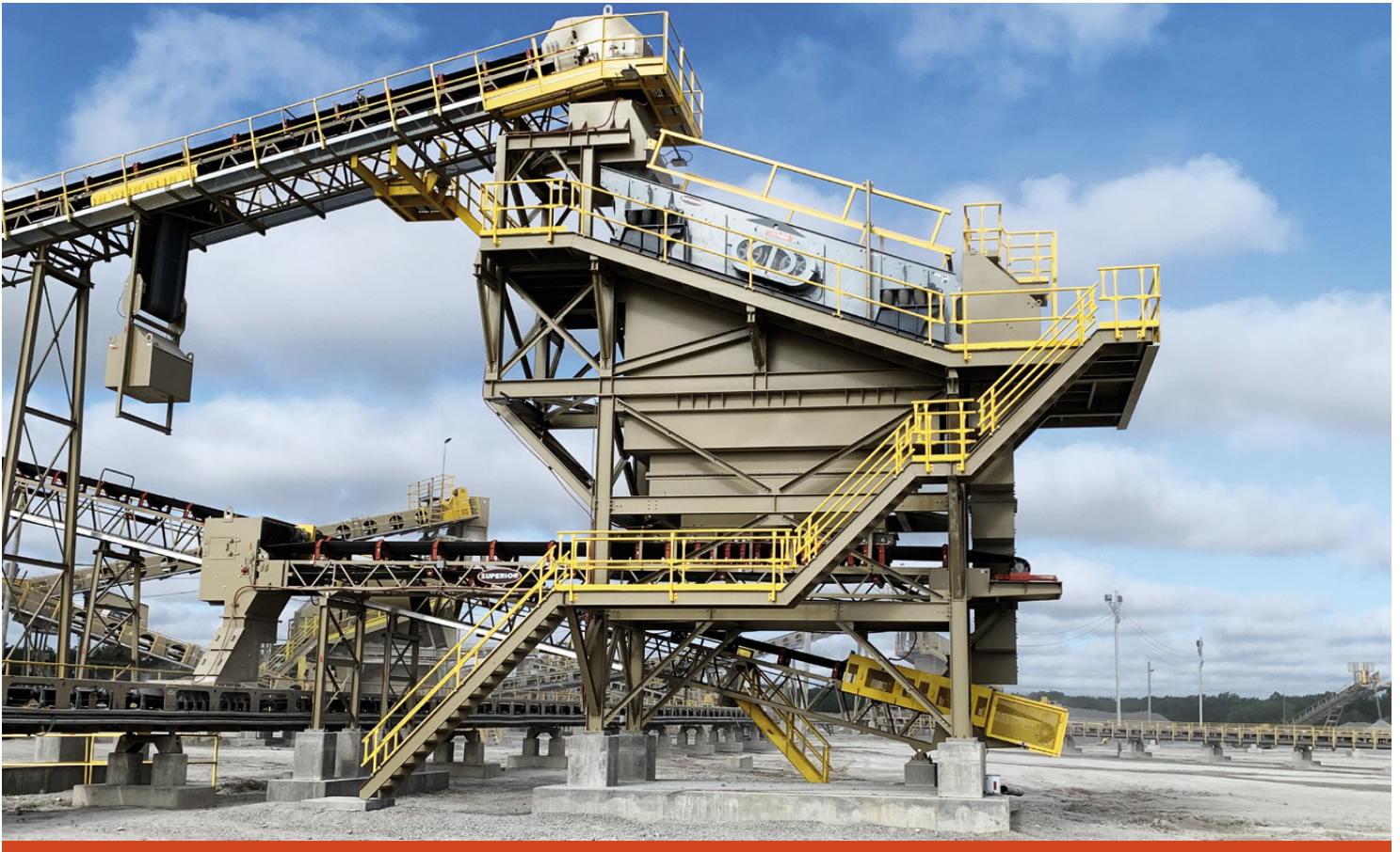
Pictured is a Superior SI8242 Anthem Inclined Screen mounted on a Superior custom structure and conveyor.
