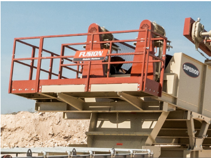
GUARDED DRIVE SYSTEM
